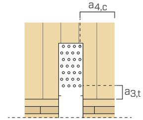
WHT PLATE T plates are designed for different floor thickness values including resilient acoustic profile. The positioning notches, as an assembly aid, indicate the maximum permitted distance (D) between the CLT wall panels in compliance with the minimum distances for HBS PLATE Ø8 mm screws. This distance includes the space required for the acoustic profile housing ( $s_{acoustic}$ ).
