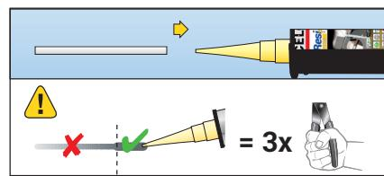
4. Attach the mixing nozzle extension MDV to the mixing nozzle MD.
