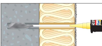
5. Fill at least 2/3 of the drill hole with composite mortar (start from the beginning). For number of strokes see mounting instructions at [www.celofixings.com](http://www.celofixings.com).
