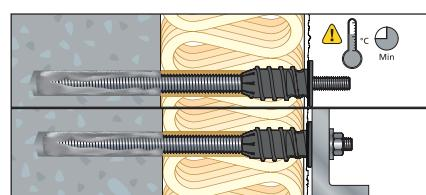
7. Observe curing time of the injection system, see cartridge label of the ResiFIX injection mortar.
