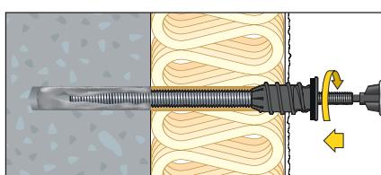
6. Screw in the ResiTHERM® 16 with the hexagon bit (included) and a cordless screwdriver until the seal is pressed against the plaster.
