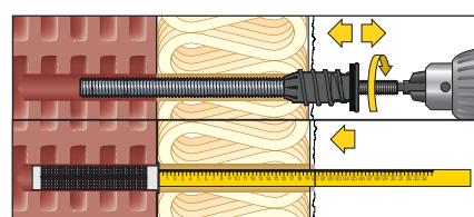
4. Enlarge the opening in the plaster for the collar of the plastic sleeve to 26 mm. To do this, briefly screw the thermal separation module in and out through the plaster for only approx. 2 thread turns or ream the plaster with a drill or drill with a bigger 26 mm drill.
