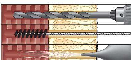
1. Drill a hole: Drill hole diameter = 20 mm.
