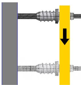
**Maximum shear loads V<sup>1)</sup> at max. 3 or 5 mm displacement if the free outer end of the ResiTHERM® 16 is not freely rotatable (e.g. connected double fixing) at 24°C/40°C<sup>2)</sup>**
