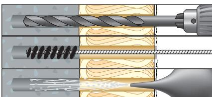
1. Drill a hole: Drill hole diameter = 18 mm
