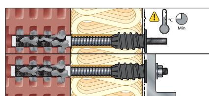
9. Observe curing time of the injection system, see cartridge label of the ResiFIX injection mortar.
