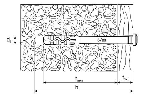
Intended use: anchorage of profiles for ETICS in concrete and masonry.
