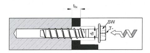
Install the screw anchor by impact screwdriver or torque wrench
